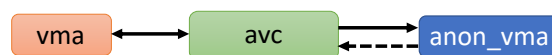
Figure 6.15: The relationship between vma , anon_vma and anon_vma_chain ( avc ). A dashed arrow indicates that anon_vma does not hold a direct pointer to the avc , but holds a reference to a red-black tree that in turn has a pointer to the avc .
