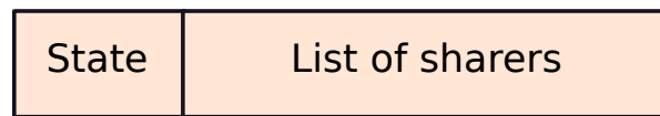
Figure 9.46: Structure of a directory entry. The tag part of the block address is not shown.
